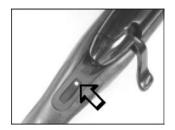
Turn bolt handle 70° upwards to unlock the bolt. Pull bolt all the way to the back by the bolt handle.
