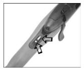
Depress the bipod arm release on the bottom of the stock and swing the bipod arms downward and forward until an audible click is heard and the bipod arms are locked in the extended position.
