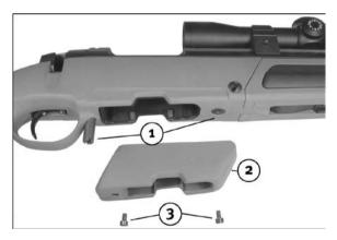
Slip on HC- adaptor (2) to the screws (1), ensure correct alignment. Turn in screws (3) and tighten it with a torque wrench (7 Nm).
