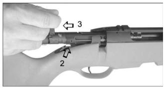
3. Hold bolt by the bolt handle and extract it from the receiver.
