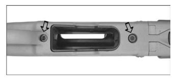
If these screws are loosened, they have to be retightened again with a torque wrench (7 Nm).
