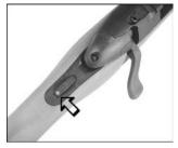
By retracting the bolt, the spent cartridge shell will be extracted and ejected. Moving the bolt forward will feed a new cartridge into the cartridge chamber of the barrel. Relock the bolt by turning the bolt handle. Move rotary safety back to position "Safe".
