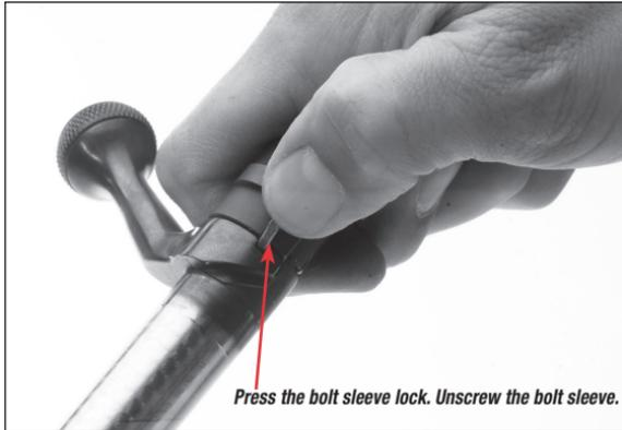
3. Raise the bolt handle and remove the bolt from the rifle as explained previously.
