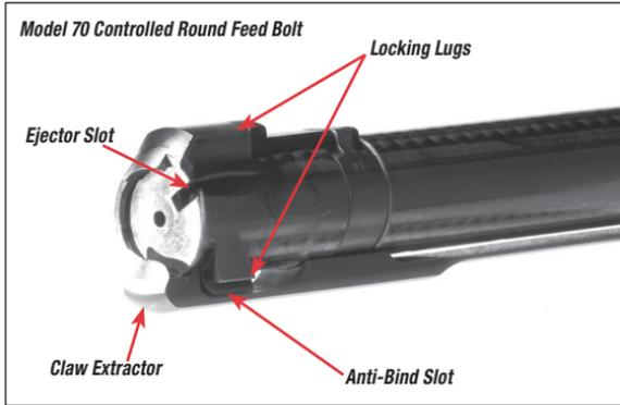
The Controlled Round Feed bolt design is a big part of the Model 70 legacy. Its massive claw extractor (Figure 1) secures approximately  $\frac{1}{4}$  of the cartridge base and fully controls the cartridge as it enters the chamber. This design also allows the cartridge to be extracted even if it is not fully chambered.
