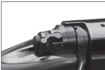
*The Model 70 three-position "safety" (left) has been proven popular by hunters and shooters for over 50 years — it blocks the firing pin and lets you open the bolt with the "safety" on.*
