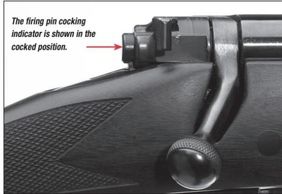
The “safety” can be operated only when the firing pin is cocked. To cock the firing pin, lift up on the bolt handle and then return it to the locked (fully down) position. When the firing pin is cocked, an indicator is visible at the rear of the bolt (Figure 7). If the indicator is protruding from the bolt sleeve a minimum of  $\frac{1}{8}$ ”, the firing pin is cocked. The “safety” can be easily operated with the thumb.
