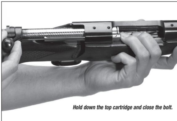
*Hold down the top cartridge and close the bolt.*
