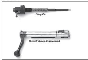
Carefully wipe clean and very lightly oil the assembly. Aerosol lubricants are excellent for forcing out any dirt, grit or moisture.
