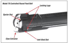
The Controlled Round Feed bolt design is a big part of the Model 70 legacy. Its massive claw extractor (Figure 1) secures approximately ¼ of the cartridge base and fully controls the cartridge as it enters the chamber. This design also allows the cartridge to be extracted even if it is not fully chambered.
