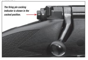
The "safety" can be operated only when the firing pin is cocked. To cock the firing pin, lift up on the bolt handle and then return it to the locked (fully down) position. When the firing pin is cocked, an indicator is visible at the rear of the bolt (Figure 7). If the indicator is protruding from the bolt sleeve a minimum of  $\frac{1}{8}$ ", the firing pin is cocked. The "safety" can be easily operated with the thumb.
